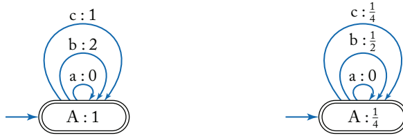
FIGURE 3.10: The figure on the left indicates the count of the parse of S = \langle bbc \rangle through \mathcal{M} and the figure on the right indicates the probabilities obtained after normalization.
